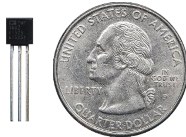
Figure 12. TMP Sensor. Quarter for scale [4]
